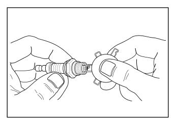
Figure 31. Checking Spark Plug Gap
